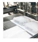
The high-performance PRINCIPAL high-level palletizer is equipped with an empty pallet magazine and an outfeed system. A bag flattener or square roller conveyor ensures that the bags are "in good shape" for stacking.
